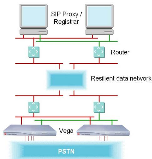
For a resilient hardware architecture, each element in the system must be duplicated, and connectivity replicated so that loss of any single component does not affect the capability of the whole system.
