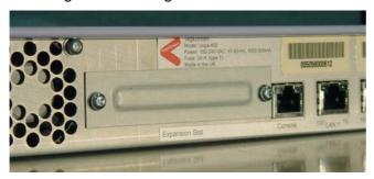
Once the Vega 400 is powered off, on the rear of the Vega 400 remove the screwed down metal cover that protects the two PCMCIA slots.
