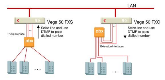
Note that if calls are presented at the PBX's trunk interface, (as it is an FXO interface) it cannot receive dialed digits, so calls will either be routed to the operator, or an auto-attendant.
