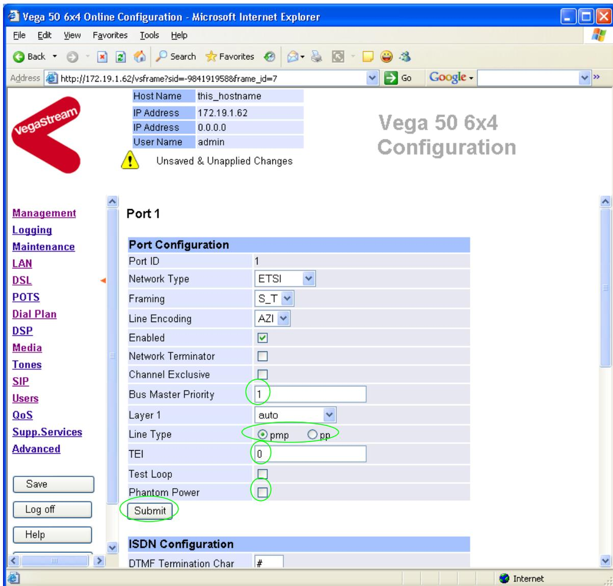
*Bus Master Priority needs to be configured so that the Vega chooses and appropriate TE trunk to synchronise its internal clock from. The priority set up will be trunk 1 is preferred clock source and trunk 3 is secondary clock synchronisation source.*
