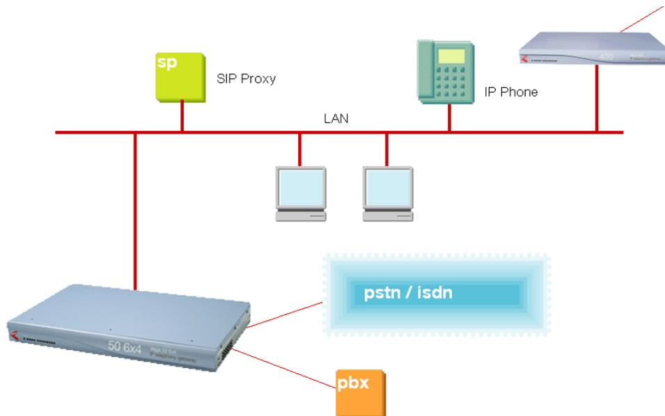
Although the Vega 50 6x4 supports two LAN interfaces, in this example configuration, only one LAN interface, LAN 1 will be used.
