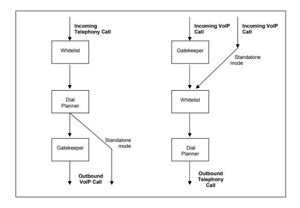
To select the mode of operation configure h323.gatekeeper.enable on the CLI or select the appropriate Gatekeeper Mode or Standalone Mode button on the h.323 page on the web browser interface.
