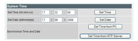
Time can be configured manually by typing in the values hh, mm and ss (in 24hr clock format) and then pressing Set Time, and the date by typing in the values in dd, mm and yyyy format and then pressing Set Date.
