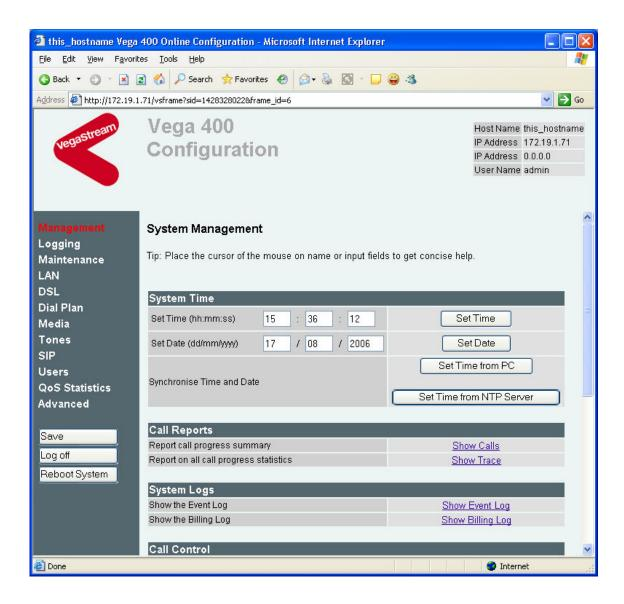
Values can be configured on the web pages by entering the value in the appropriate text box and then pressing the appropriate Set Time Set Date Submit or Apply button adjacent to or immediately below the section being changed.
