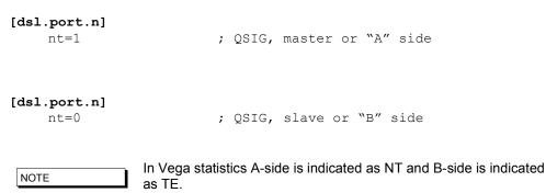
When configuring A-side and B-side, the value of the  $clock\_master$  parameter should also be checked.
