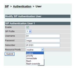
The resource priority is configured through the selection of an entry in a pull down box. The values contained in the pull down box are the values defined in the NameSpace configuration (see section 15.6.1 "Configuring NameSpace for").
