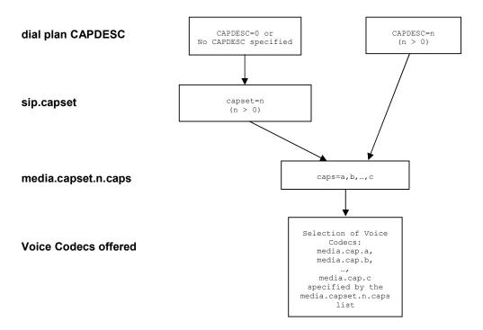
In the dial planner a token CAPDESC: can be used (in a dest statement where the interface is IF:9901) to specify which codec set (media.capset.n.caps list) is to be used to specify the list of codecs to offer (and their priority order).
