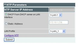
The Vega can either pick up the IP address of the NTP server from a DHCP server (in which case you need to select whether the DHCP server to get the NTP IP address is accessed via LAN interface 1 or LAN interface 2) or a static IP address for the NTP server may be configured.
