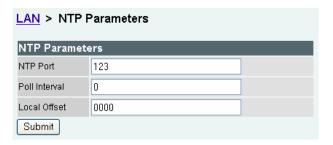
The value for Local Offset is either in HHMM or for negative offsets -HHMM format.
