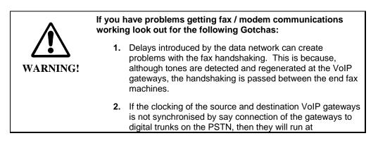
independent clock speeds. Over time, internal buffers will overflow or underflow due to the difference in clock (data) rates. This will cause the fax machines / modems to have to re-negotiate. If the slip is too great then re-negotiation will take more time than data transmission time and connections are likely to fail.
