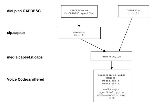
In the dial planner a token CAPDESC: can be used (in a dest statement where the interface is IF:9901) to specify which codec set (media.capset.n.caps list) is to be used to specify the list of codecs to offer (and their priority order).
