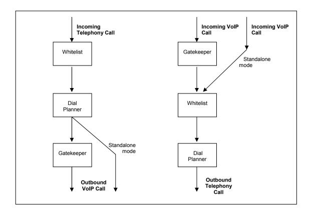
To select the mode of operation configure h323.gatekeeper.enable on the CLI or select the appropriate "Gatekeeper Mode" or "Standalone" button on the H.323 page on the web browser interface.
