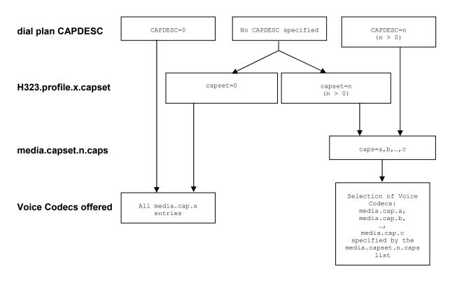
In the dial planner a token CAPDESC: can be used (in a dest statement where the interface is IF:0501) to specify which codec set (media.capset.n.caps list) is to be used to specify the list of codecs to offer (and their priority order).
