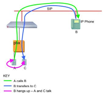
The Vega's default behaviour relies on detecting that two SIP call legs have the same call ID in order to initiate the QSIG side un-tromboning. Other headers can be checked and verified using the following two parameters:
