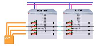
The status of the ISDN fallback relays can determine whether SIP registration takes place on a Vega 400 (models where ISDN fallback relays are fitted).
