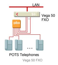
To understand the capabilities of each it is useful to think of the Vega 50 FXS being like an 8 port PBX and the Vega 50 FXO being like a bank of 8 virtual telephones.
