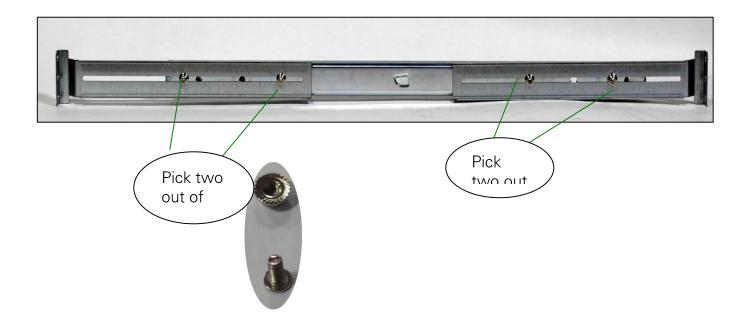
**Note**: You will only need to secure "two" out of these four screw holes for each L-shaped bracket to mount the outer rail safely. Extra holes are for compensating different mechanical designs.
