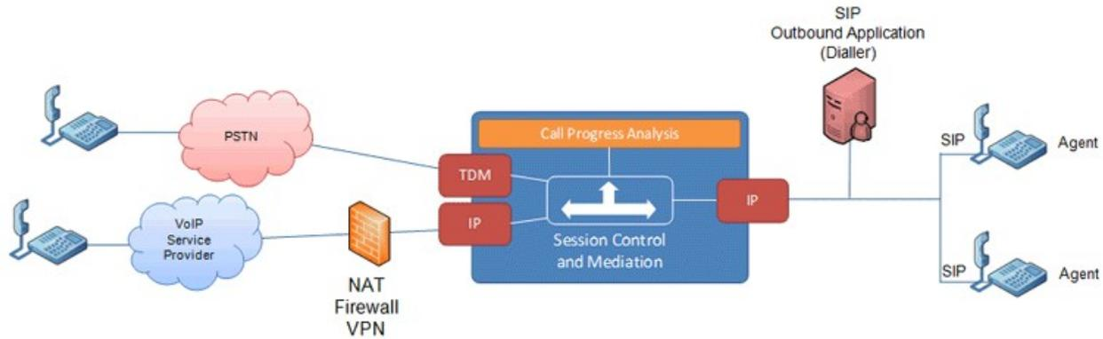
Note that the application provides connectivity to both legacy and IP networks, and routes both inbound and outbound traffic through a single element.
