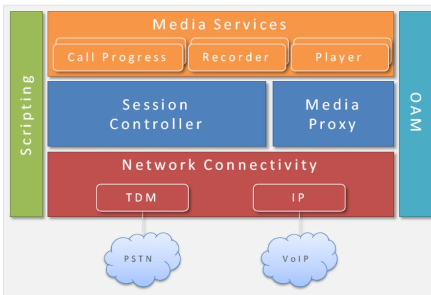
Each software subsystem has its own *OAM (Operations, Administration, and Maintenance)* components, for increased flexibility and manageability.
