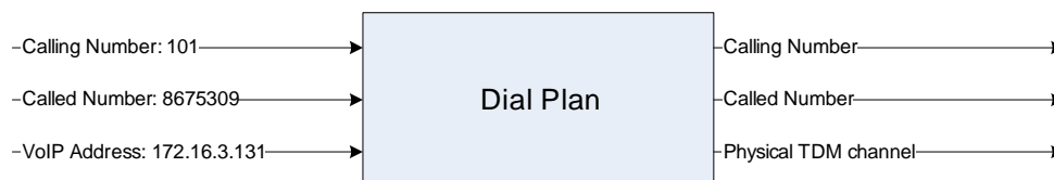
Figure 22. VoIP to TDM calls
