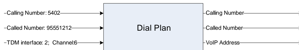
Figure 23. TDM to VoIP calls
